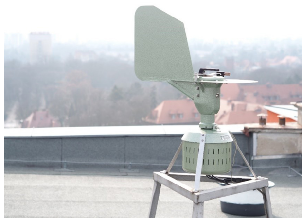
Fig. 8. Hirst-type pollen trap located at the studied site (dormitory Eskulap)
